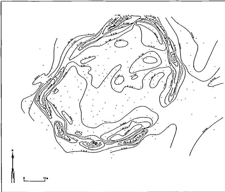
Fig. 9. Magnetometric map of Broborg, same area as shown in Fig. 2. Points of measurement marked by dots. Contour intervals 100 nT, screened areas > 51200 nT.
