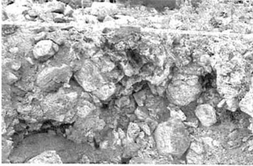
Fig. 12. Front of trench *a-a'* (Fig. 2), about half-way through the vitrified layer. Vitrification is found at the top 30 cm layer, underlain by fire-cracked gneissic granite.
